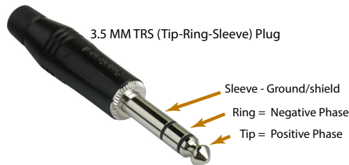
Figure 2-8: 3.5 MM TRS Connections
