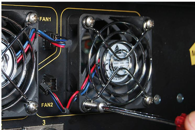
2. Insert the connector into the adjacent receptacle.
