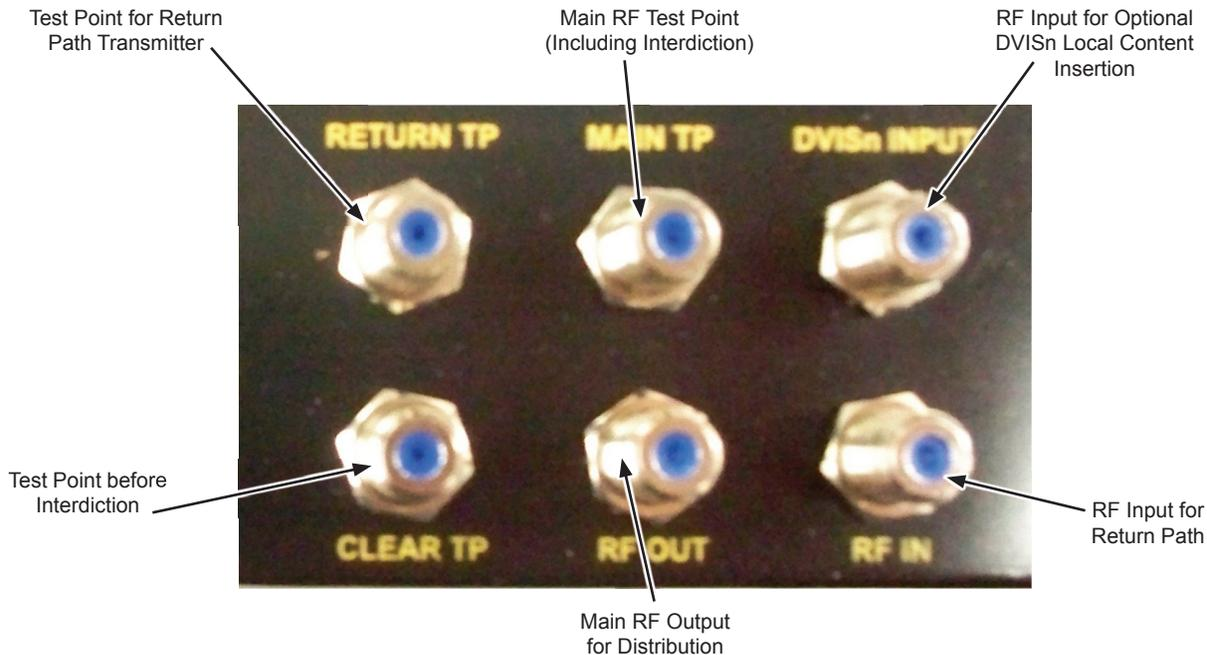
Figure 3: RF Connections
