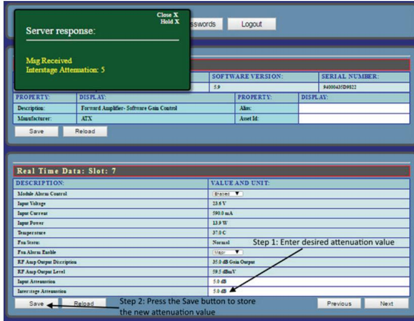
Figure #7: Interstage Attenuation Electronic Control
