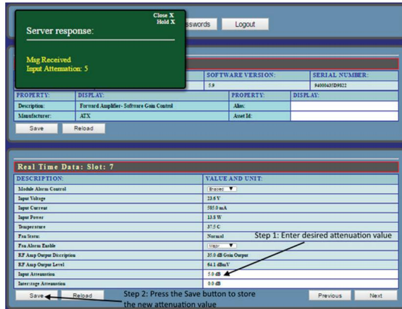
Figure #5: Input Attenuation Electronic Control
