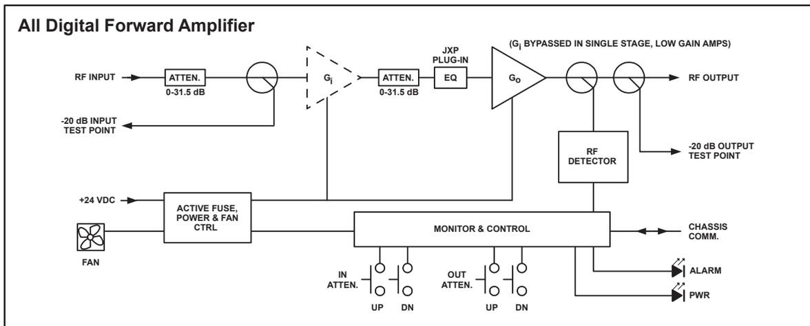
Figure #3: All Digital Forward RF Amplifier Functional Diagram
