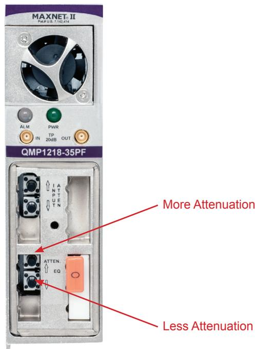
Figure #8: Push Button Location for Interstage Attenuation
