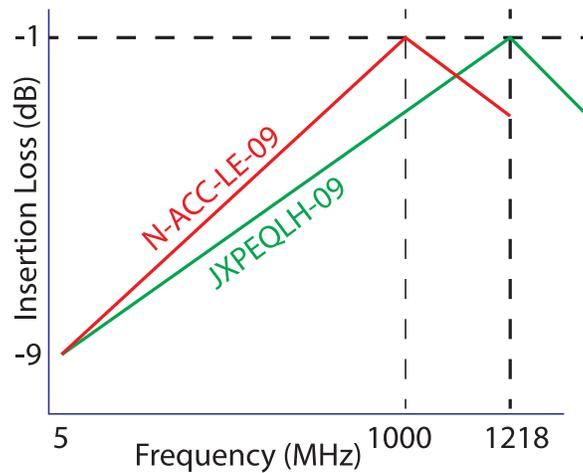
**Figure #10: Example Difference of 1 GHz vs 1.218 GHz Models. Both are 9 dB Linear Equalizers.**
