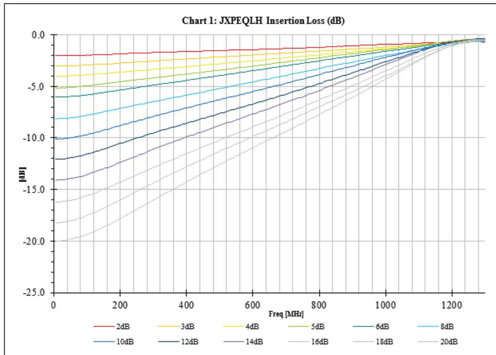
Figure #11: Typical Plot JXPEQLH with Different EQ Values
