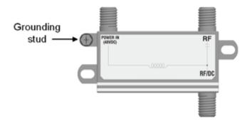
d. Attach a ground wire to the grounding stud on the power inserter/filter module housing. Insert the bare end of a protective earth (PE) ground wire, AWG 18 or larger, under the grounding screw on the unit, and then tighten the screw from 18 in-lb to 20 in-lb (2.0 Nm to 2.3 Nm).
